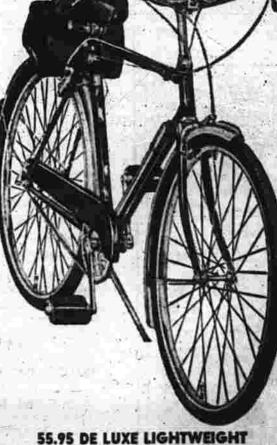
America's heart. Fully equipped with 3-speed shift, Caliper brokes, generator, headlamp and tail light. Bright chrome fenders. Tire pump and tourist bag, too.
